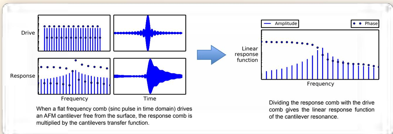
Probing nonlinear response with a frequency comb is particularly advantageous. **Intermodulation** or frequency mixing of multiple tones in a drive comb generates many new frequencies in the response at integer multiples of  $\Delta f$ . Measuring multiple amplitude and phase response at mixing frequencies is a powerful new paradigm for understanding nonlinear systems [3].
